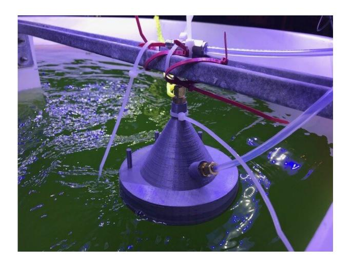
A new technology developed at UC San Diego uses chemical ionization mass spectrometry to alert algae growers when volatile gas signatures change, allowing them to harvest algae crops when under attack by contaminating organisms. Credit: UC San Diego
