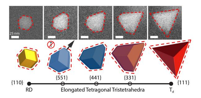
An illustration shows the progression of a gold seed to a crystalline, asymmetrical tetrahedron nanoparticle. The images were captured at Rice University through a technique known as liquid cell transmission electron microscopy. Credit: Jones Research Group/Rice University
