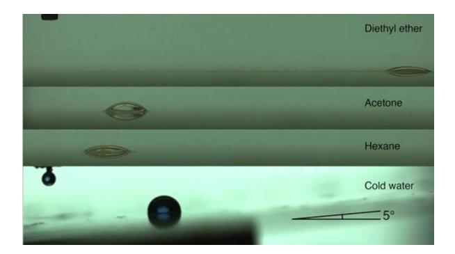
When a cold/hot or volatile droplet is liberated on a lubricated piezoelectric crystal (lithium niobate) at ambient temperature, the droplet instantaneously propels for a long distance. Credit: The University of Hong Kong
