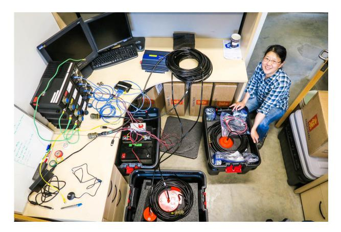
Dr. Sato with echosounder equipment used to detect fish from onboard ship. Credit: A.W. Trites, University of British Columbia
