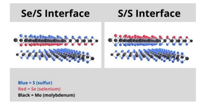
The two types of interfaces between layers of transition metal dichalcogenides (TMD) 2D materials where the top layer is a Janus TMD with two types of atoms (selenium and sulfur) and the bottom layer is a regular TMD with one type of atom (sulfur). The S/S interface is much stronger than the Se/S interface due to the charge distribution from the imbalance in S atoms. Credit: Penn State Materials Research Institute
