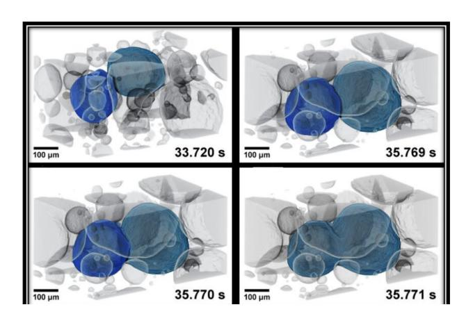
Such metal foams based on aluminum alloys are being investigated as lightweight materials, for example for the construction of electric cars. The morphology, size and cross-linking of the bubbles are important to achieve the desired mechanical properties such as strength and stiffness in large components. Credit: *Advanced Materials / PSI / HZB*
