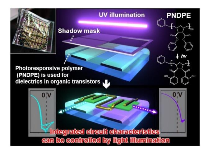
Figure 1: Schematic showing the process that allows for precise control of the organic transistor characteristics using light irradiation. The inset displays a photograph of the final device. Credit: Takafumi Uemura et al.
