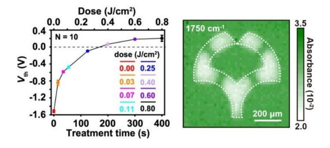
Figure 2: (Left) Relationship between the light illumination (dose) and the threshold voltage (Vth) for the organic transistors. (Right) FTIR microscopy image showing the two-dimensional spatial distribution of the molecular structure alteration. Certain regions were partially irradiated to create the Osaka University logo, with an estimated spatial resolution of ~18  $\mu$ m. Credit: Takafumi Uemura et al.
