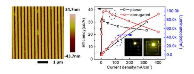
Tunable SPP resonance in OLEDs based on corrugated alloy electrodes. Credit: Compuscript Ltd
