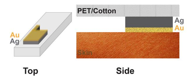
A diagram of the bioelectrical sensor, showing the gold (Au) and silver (Ag) layers attached to fabric and making good contact with the skin. Credit: Taehwan Lim
