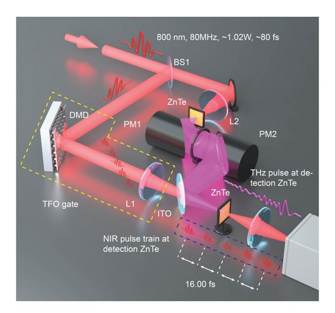
Schematics of the experimental setup showing a temporal fan out (TFO) gate
