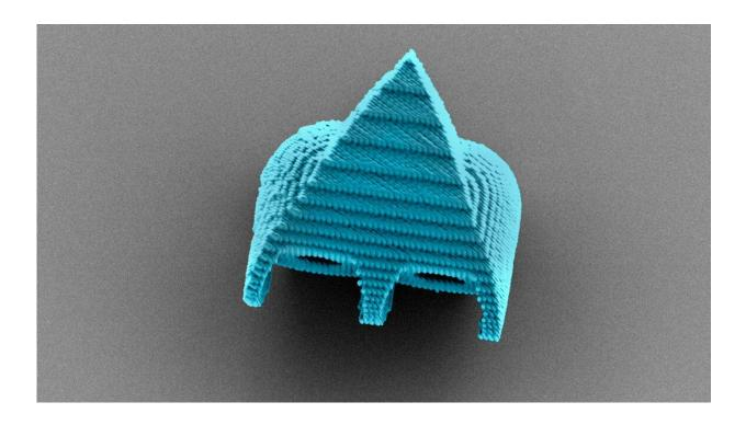
A scanning electron microscope image shows a cell-size robotic swimmer that can be powered and steered by ultrasound waves. Credit: Cornell University
