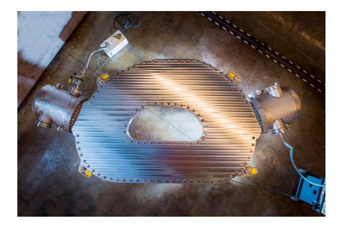
This large-bore, full-scale high-temperature superconducting magnet designed and built by Commonwealth Fusion Systems and MIT's Plasma Science and Fusion Center (PSFC) has demonstrated a record-breaking 20 tesla magnetic field. It is the strongest fusion magnet in the world. Credit: Gretchen Ertl, CFS/MIT-PSFC, 2021
