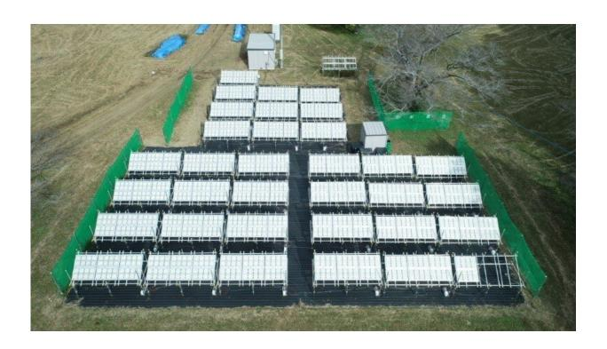
Panoramic view of the hydrogen production photocatalytic panel reaction system. Credit: Adapted from Nishiyama, H., Yamada, T., Nakabayashi, M. et al.
