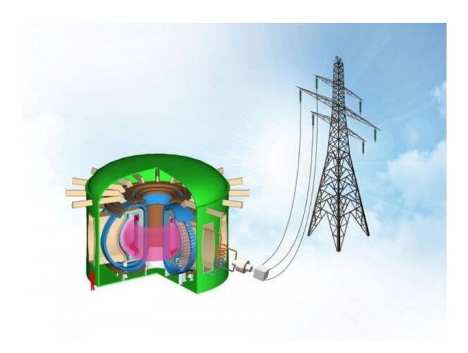
The Compact Advanced Tokamak (CAT) is a potentially economical solution for fusion energy production that takes advantage of advances in simulation and technology. Credit: Image courtesy of General Atomics. Tokamak graphic modified from F. Najmabadi et al., The ARIES-AT advanced tokamak, Advanced technology fusion power plant, Fusion Engineering Design, 80, 3-23 (2006).
