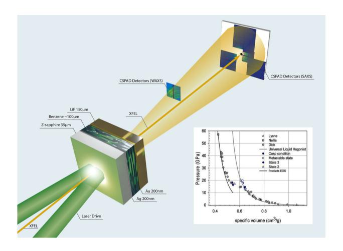
Experimental configuration of laser-driven shock compression experiments on benzene. Credit: Los Alamos National Laboratory
