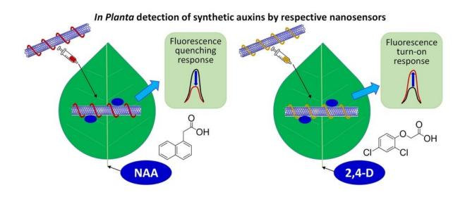
Nanosensors developed at the Singapore-MIT Alliance for Research and Technology (SMART) can detect synthetic auxin plant hormones NAA and 2,4-D. Credit: Singapore-MIT Alliance for Research and Technology
