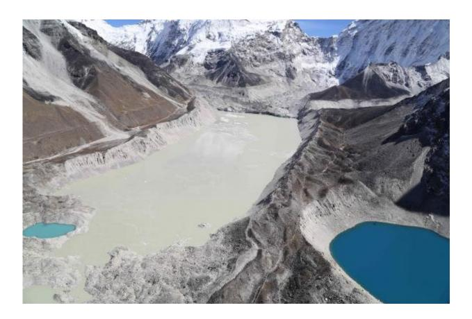
Imja Lake, Nepal, is considered one of the most hazardous lakes in Nepal. The moraine dam at lower left was engineered in 2016 to reduce the lake level slightly and to stabilize the outlet river so as to slightly reduce the glacial lake outburst flood (GLOF) hazard. A hazard early warning system is arranged downstream. Credit: Jeffrey S. Kargel, 2016.
