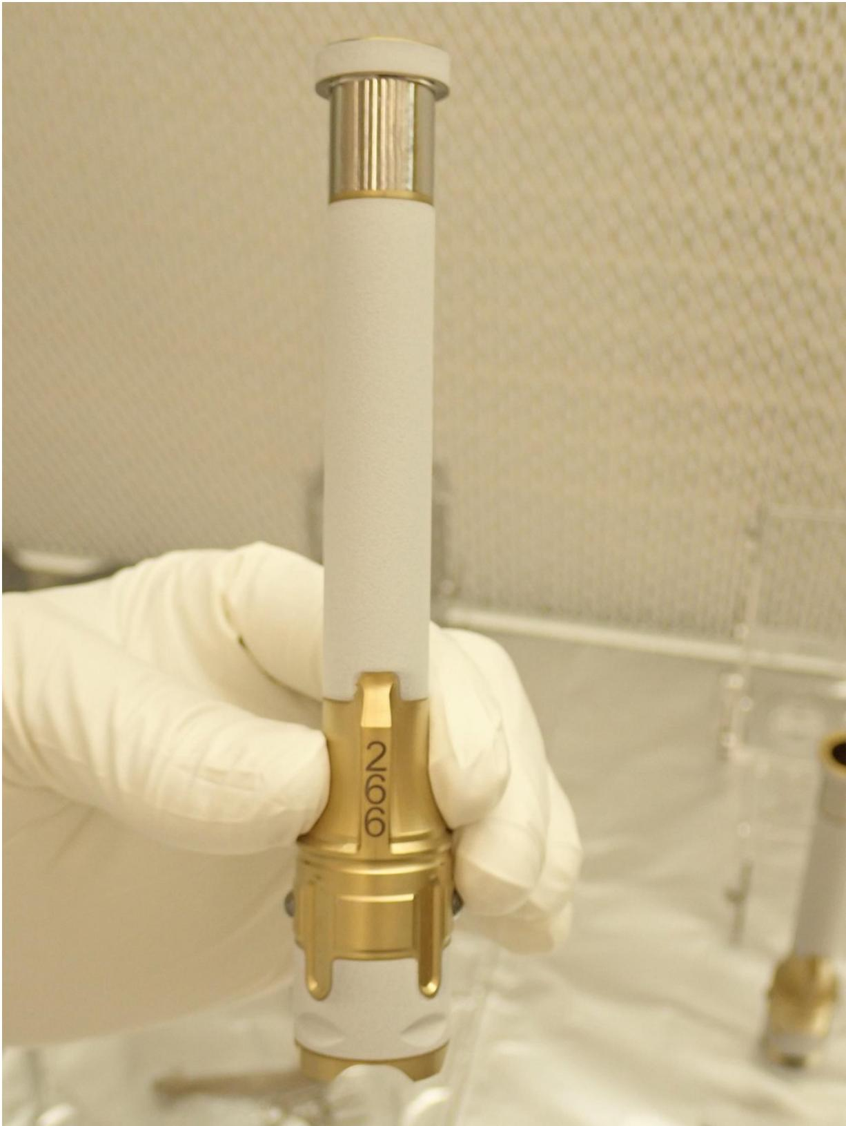
Sample tube number 266 was used to collect the first sample of Martian rock by NASA's Perseverance rover. The laser-etched serial number helps the scientists identify the tubes and their contents. Credit: NASA/JPL-Caltech
