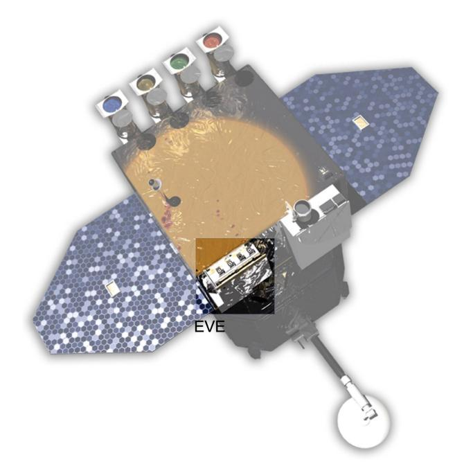
An illustration of the SDO spacecraft with the EVE instrument highlighted. Credit: NASA/SDO
