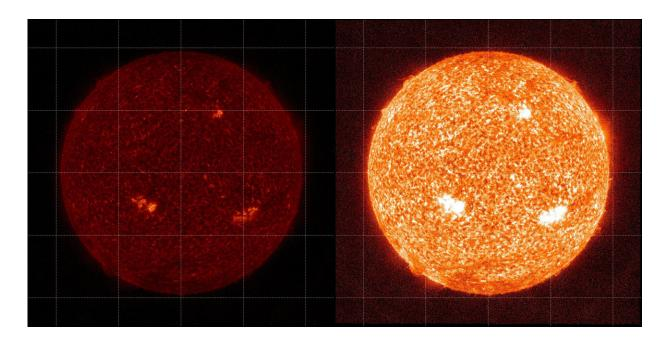
The images show the sun as seen by another SDO instrument, AIA, in 304 Angstrom light in 2021 before degradation correction (left) and with corrections from a sounding rocket calibration (right). Credit: NASA/SDO
