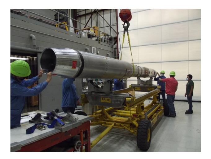
The EVE payload is loaded onto a cart for transport at the White Sands Missile Range. Credit: NASA
