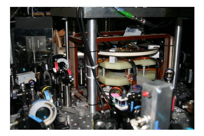
The experimental apparatus used to create ultracold RbCs molecules and perform these experiments. Credit: Gregory et al.
