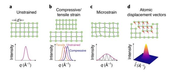
Fig. 1: Definition and measurement of strain in halide perovskites. Credit: DOI: 10.1038/s41563-021-01097-x
