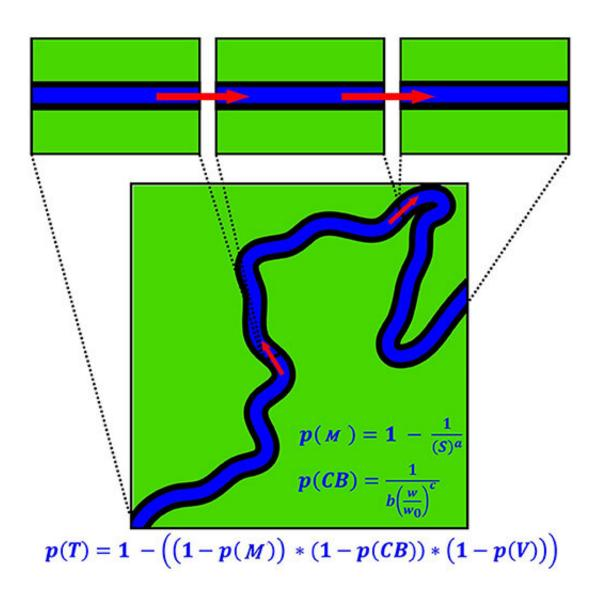
Schematic illustration of the transfer of macroplastic debris downstream from cell to cell. Also shown are the equations used to calculate the combined probability of trapping, p(T), probability of trapping along meander bends, p(M), and probability of trapping along channel banks, p(CB). Credit: DOI:
