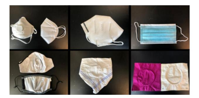
Different samples that were used in this study are shown from top right to bottom in clockwise direction: N95 respirator, KN95 respirator, surgical mask, wash/dry sample coupon, 2-ply bandana and cloth mask. Credit: Marina Vance
