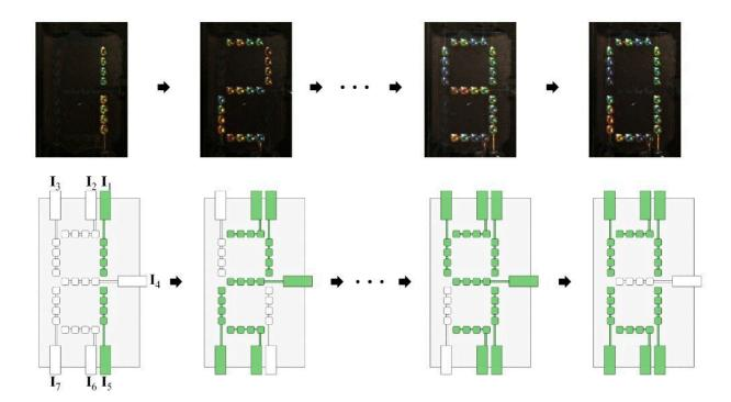
Multiple pixels can be connected to the same air pump, allowing for more complex displays. Credit: University of Pennsylvania
