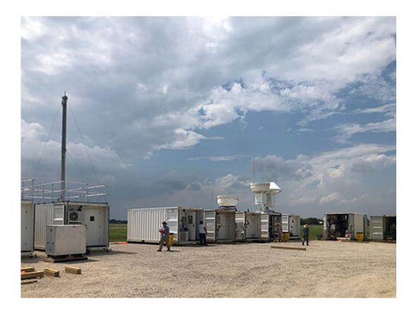
ARM team members set up the ARM Mobile Facility—a series of containers outfitted with sophisticated atmospheric and meteorological sampling equipment—at the La Porte (Texas) Municipal Airport. Equipment at this main site for the TRACER campaign will operate from October 1, 2021, through September 30, 2022. Credit: ARM
