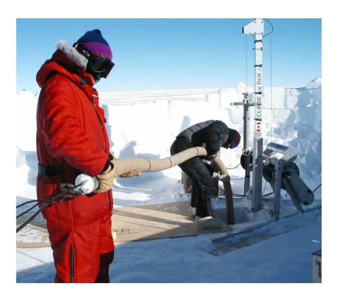
Researchers insert a vacuum line down a borehole in Megadunes, Antarctica, to pump air out of the snow pack. Researchers at UCI analyzed the "firn" air to determine that the amount of molecular hydrogen in Earth's atmosphere has
