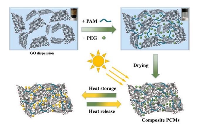
Schematic diagram of the PEG/GO-PAM composite PCMs synthesis. Credit: LI Yangeng
