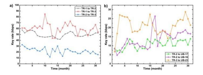
The key rates versus time for some representative links. (a) The key rates between the three trusted relays. (b) The key rates between trusted relay and user. In the robustness test, 11 user nodes have continuously run for 31 months. The key rates are recorded every 30 s and taken average over a month. The detailed key rates are given in Supplementary Tables V and VI. Credit: Nature Quantum Information, 10.1038/s41534-021-00474-3
