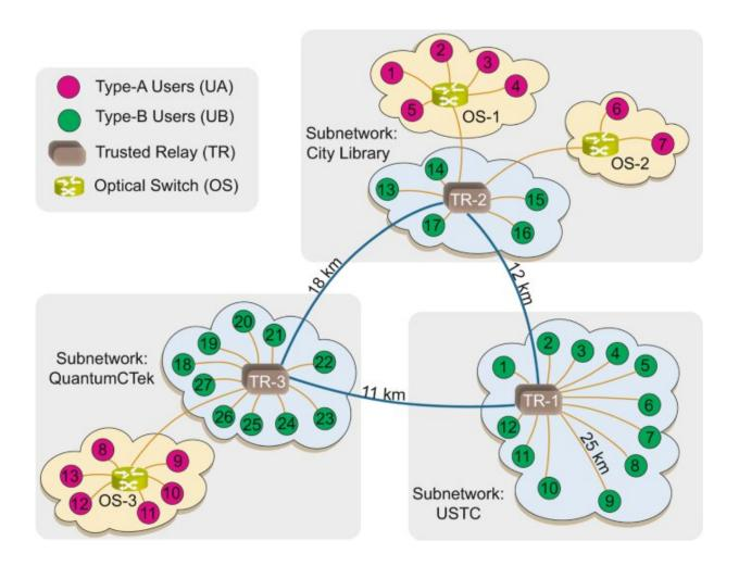
The topological structure of our quantum network. The network mainly comprises three subnetworks that are directly connected to each other. In each subnetwork, there are multiple users connected to intermediate nodes in different ways, either by an all-pass optical switch (OS) or by a trusted relay (TR). Users connected by a switch are denoted as red dots (Type-A Users, UA),
