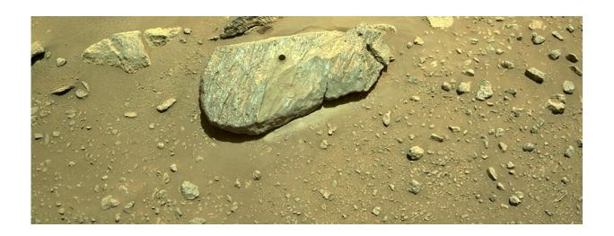
In this image released by NASA, the drill hole from Perseverance's second sample-collection attempt can be seen in a rock, in this composite of two images taken on September 1, 2021 by one of the rover's navigation cameras.
