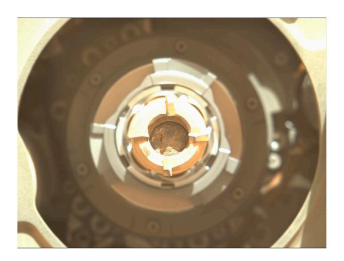
This Wednesday, Sept. 1, 2021 photo made available by NASA shows the first rock sample for return to Earth, obtained by the Mars Perseverance rover. A month ago, Perseverance drilled into much softer rock, and the sample crumbled and didn't get inside the titanium tube. The rover drove a half-mile to a better sampling spot to try again. Team members analyzed data and pictures before declaring success. Credit: NASA/JPL-Caltech/ASU via AP
