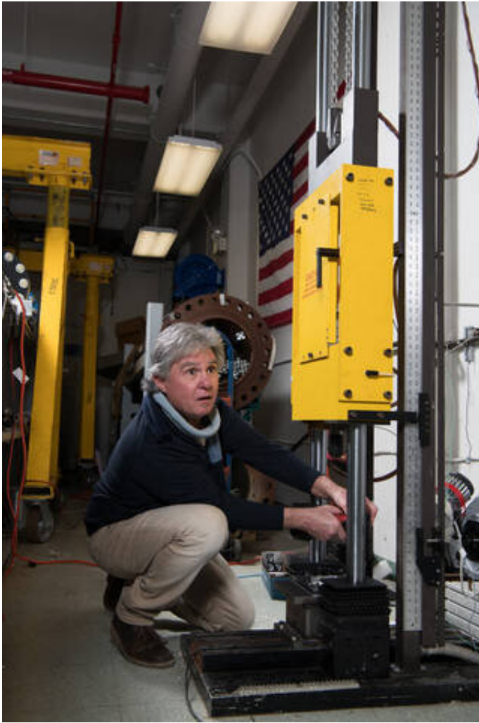
Ballistics Lab technical lead Mike Pereira sets up a drop test. Credit: NASA
