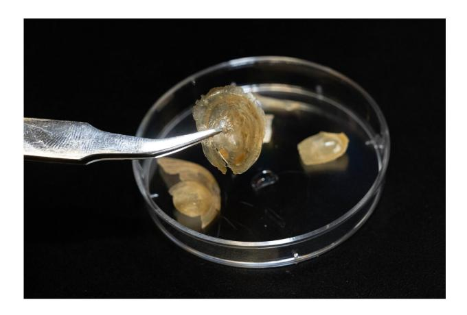
The shell of the brachiopod Discinisca tenuis is hard and brittle but becomes soft and flexible when exposed to water. Credit: Brookhaven National Laboratory
