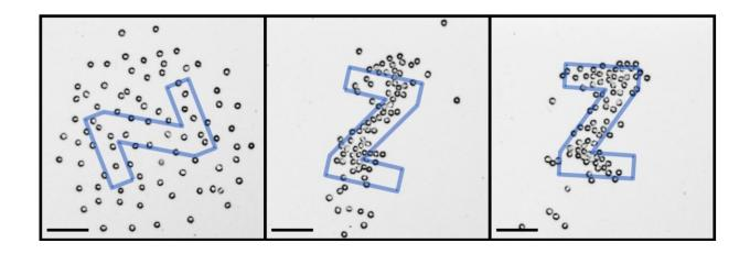
Snapshots of a shape formation experiment showing several stages of the process, from the initial particle distribution to the end result. Credit: Artur Kopitca/Aalto University
