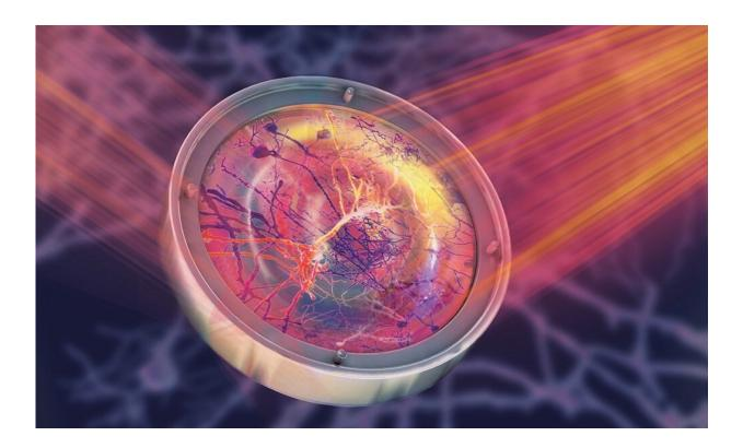
A deformable mirror used in microscopy to focus light within live tissues. They would normally distort its propagation. Thanks to this mirror, we can see clear and crisp images of neuronal cells deep inside the brain. Credit: Isabel Romero Calvo/EMBL
