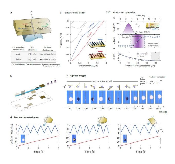
A, Driving locomotion of a rectangular plate on a frictional surface through excitations of elastic waves by pulsed optical absorption. Table: relationships
