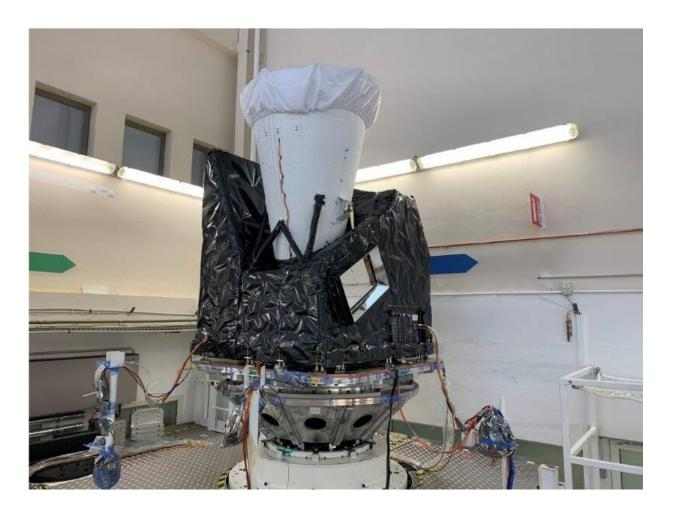
The Flexible Combined Imager, developed by Thales Alenia Space, has undertaken an extensive system and environmental test campaign, which concluded with the complex 'Optical Vacuum' performance testing. In this photo, the instrument is undergoing mechanical testing. Credit: Thales Alenia Space
