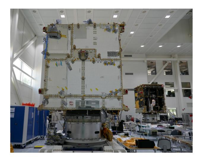
The high stability three axis stabilised platform, developed by OHB in Bremen, has undertaken extensive system testing demonstrating the platform's performances and associated data handling links with the instruments. Credit: Thales Alenia Space
