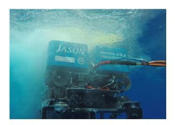
Jason II, a remotely operated robot submarine connected by cable to the ship, was used to collect the rock samples from the seafloor. Credit: Lucas Kavanagh
