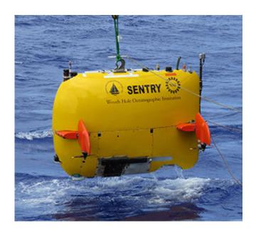
The Sentry, an autonomous undersea vehicle, was used to map the magnetic stripes in Pito Deep, a large chasm in the Pacific Ocean that provides a cross-section of samples of lower oceanic crust. Michael Cheadle and Barbara John, both UW professors of geology and geophysics, contributed to a paper titled "Three-Dimensional Magnetic Stripes Require Slow Cooling in Fast-Spread Lower Ocean Crust" that was published Sept. 23 in *Nature*. Credit: Michael Cheadle
