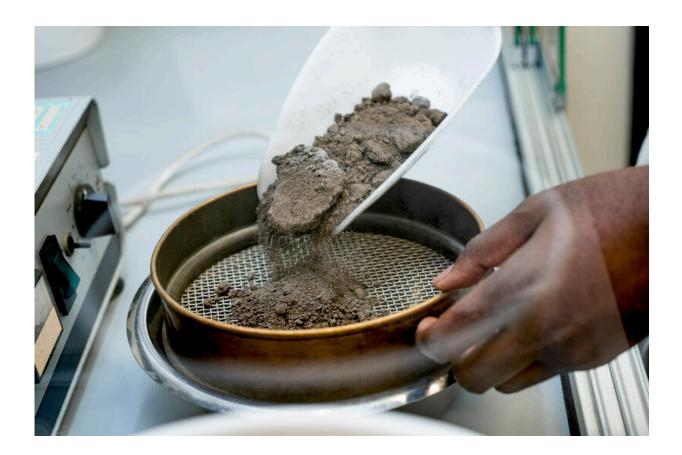
In order to investigate how the use of biochar affects the soil, it is sieved through. The meshes of the sieve measure two millimetres. Credit: Damian Gorczany
