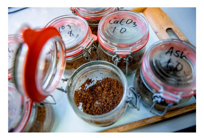
Preincubation of ash and calcium carbonate (CaCO2) treated soil for the liming experiment Credit: Damian Gorczany
