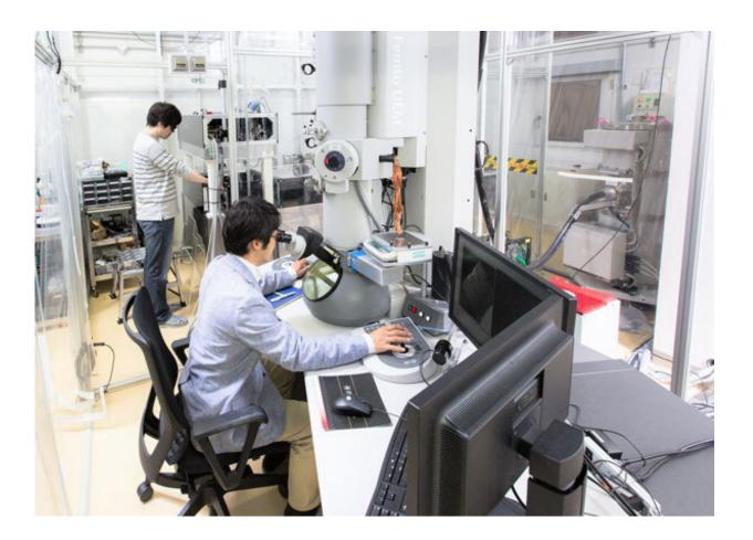
Figure 1: Takahiro Shimojima (seated) using an ultrafast transmission electron microscope to look at skyrmions in a thin film of cobalt zinc manganese. Credit: RIKEN Center for Emergent Matter Science
