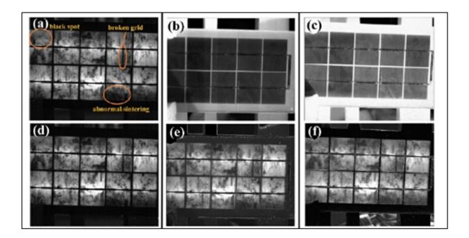
Researchers developed a new system that can detect defects in silicon solar
