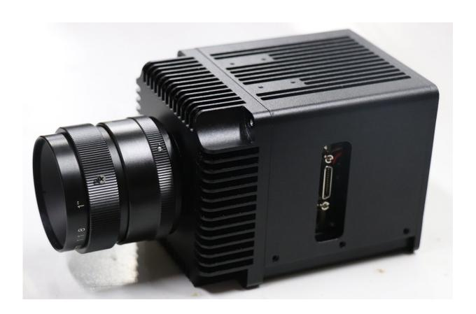
The researchers used an InGaAs detector with a very high frame rate to acquire a sequence of images of solar panels as a modulated electric current was applied. The very fast imaging speed available from this detector allowed more changes between the images in the sequence to be distinguished. Credit: Yunsheng Qian, Nanjing University of Science and Technology
