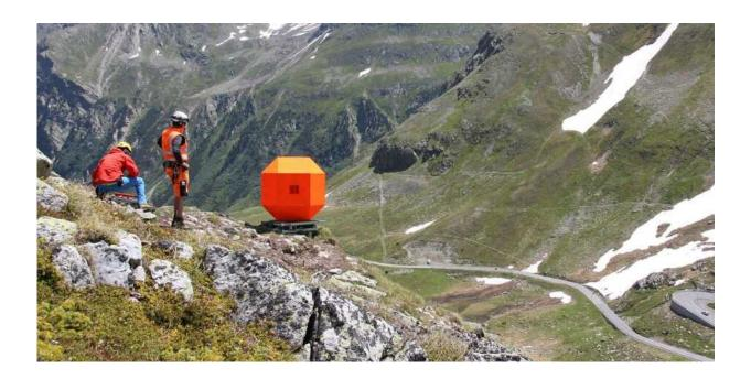
One of the concrete blocks positioned on the tilting platform that will be used to set it in motion. Credit: SLF / Martin Heggli
