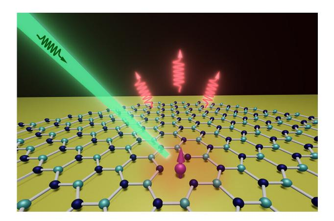
A spin qubit in a 2D material on a gold film. When placed on a gold-film microwave stripline, spin defects in hexagonal boron nitride show a record-high contrast of their optically detected magnetic resonance and simultaneous plasmonic enhancement of their photon emission. Credit: Zhujing Xu and Tongcang Li
