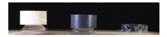
Homemade glacier. To replicate glacier table formation, cylindrical stones made of polystyrene, PVC, and granite were placed on a plate made of ice. As the ice melted, the plastics (polystyrene and PVC) formed tables because they are relatively poor conductors of heat, whereas the granite—a stronger heat conductor—sunk into the ice. Credit: M. Hénot et al.
