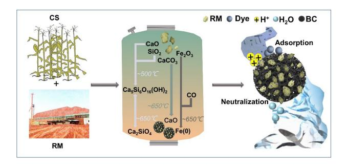
Diagram of the fabrication process and mechanism of FBCs. Credit: GAO Yujie
