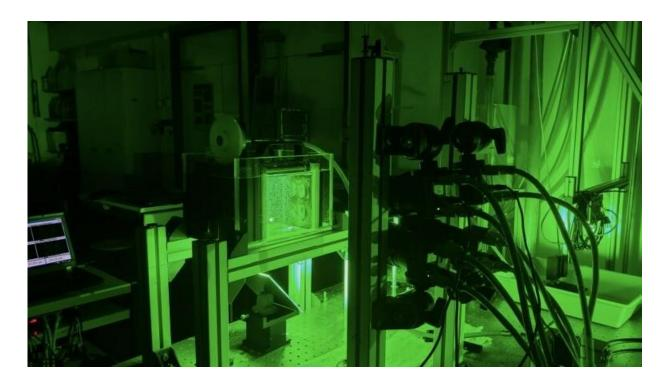
The research team from ETH Zurich generated a turbulent flow within a closed water tank and tracked the movement of fibers. Credit: ETH Zurich
