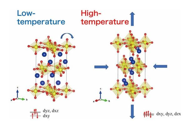
The structural distortions in  $Ca_2RuO_4$  are responsible for its anisotropic thermal expansion. Credit: Masaki Azuma from Tokyo Institute of Technology
