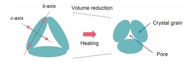
The changes observed in the material structure and NTE owing to anisotropic thermal expansion of crystal grains. Credit: Masaki Azuma from Tokyo Institute of Technology
