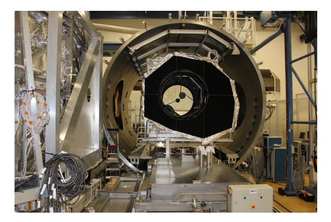
In order to prove that Euclid can accurately perform its observations, the sky was simulated in the thermal vacuum chamber to recreate on-orbit observation condition. This simulator, shown in the picture inside the vacuum chamber is a 'collimator' that projects test star sources in the Euclid telescope as if Euclid was observing them from an infinite distance like in space. Credit: ESA
