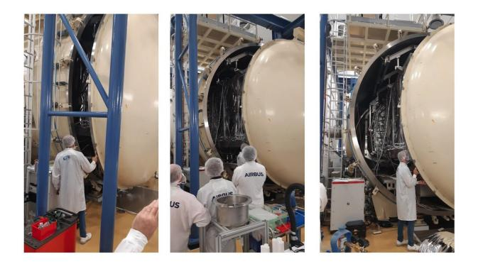
ESA's Euclid mission successfully passed tests to show that it can perform in the extreme environment of space. At Centre Spatial de Liège (CSL) in Belgium, the
