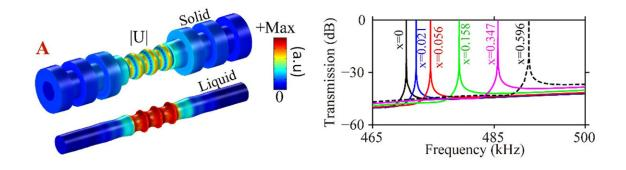
Left panel: Tubular phononic crystal (TPC) with a Fabry-Perot cavity filled with a set of propanol-water mixtures: representation of the acoustic field in the solid (up) and in the liquid (down). Right panel: Application of the sensor for the determination of the propanol-water mixtures with molar ratio x ranging from 0 to 59.6% as a function of the measured frequency (millimeter size). Credit: Yan Pennec
