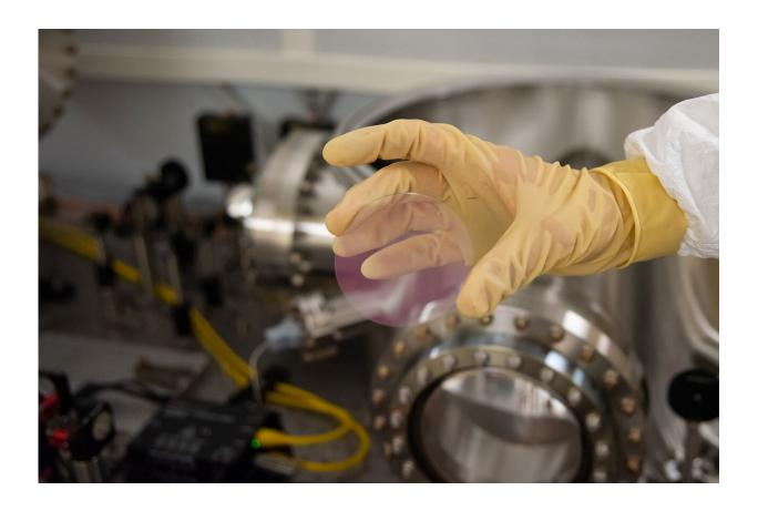
The LIGO coating materials to be tested are deposited on thin glass disks, much smaller than the LIGO mirrors. The pinkish color in the photo is due to the thin layer of metal oxide deposited on the surface. Credit: Caltech
