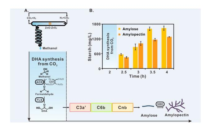
Starch synthesis via artificial starch anabolic pathway (ASAP) from carbon dioxide. Credit: TIBCAS
